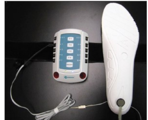
FIGURE 1. Audio biofeedback device and force transducer affixed to the rearfoot area of the shoe insole.
